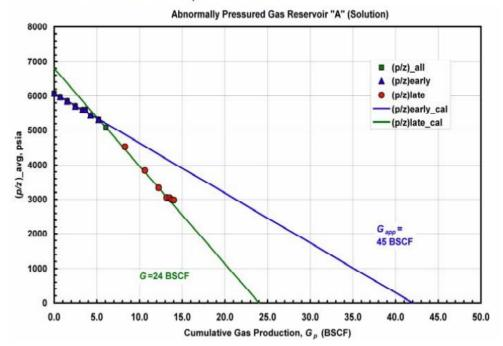
"Corrected" p/z Versus Cumulative Gas Production (G<sub>p</sub>): Reservoir "A"
